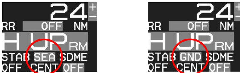
When SDME or EPFS is not available for any reason, it is possible to get the speed over ground by setting reference target.
