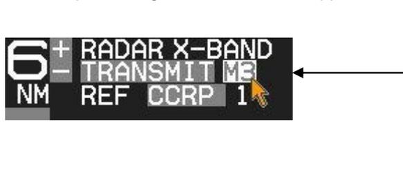
\* Pulse length can be changed directly at the upper left of the display, with CURSOR and **[ENT]** key.
